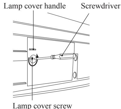
**4** Loosen the lamp unit screw with a screwdriver. Then, grasp the lamp unit as shown in the diagram, and slowly remove from the projection display.
