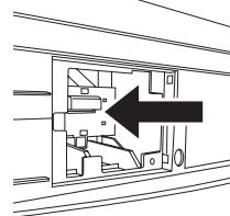
**6** Replace the Lamp unit and cover screws. Tighten the lamp unit/cover screw with a screwdriver.
